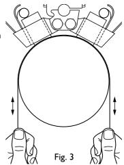
After bedding, the holders and brushes must be thoroughly cleaned. Brushing and then followed by thorough vacuum cleaning to remove all debris.
